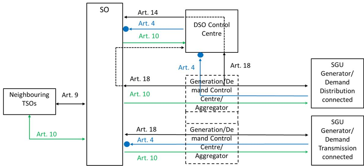
**Figure 4:** Exchange of Real Time information
