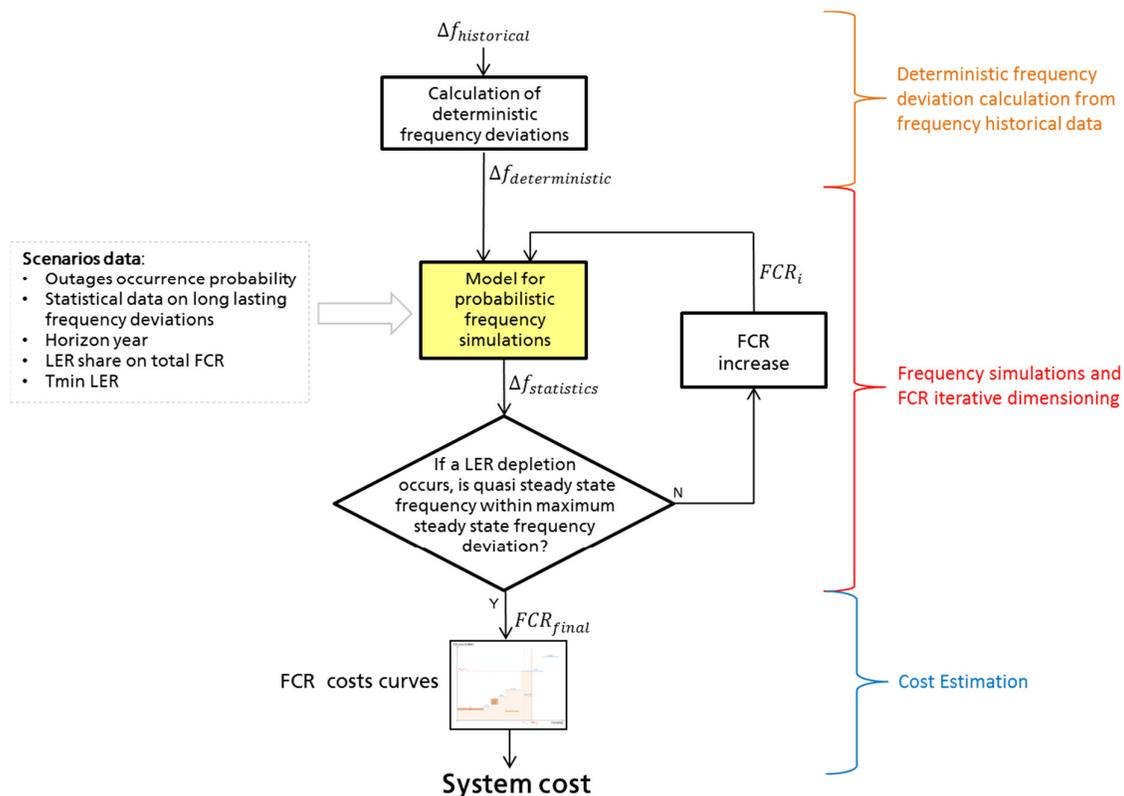
Figure 1 Process workflow
