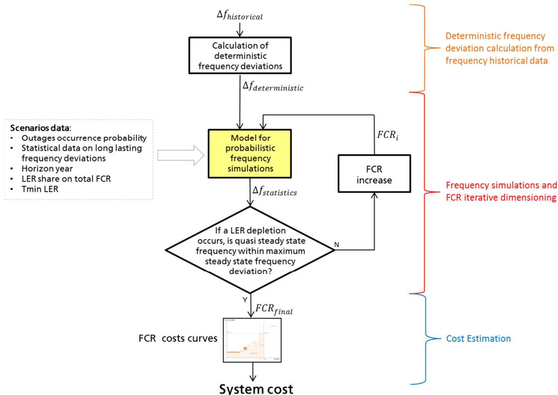
The workflow contains an iterative process in which, if the requirements on LER depletion are not fulfilled, the FCR total amount is gradually increased.
