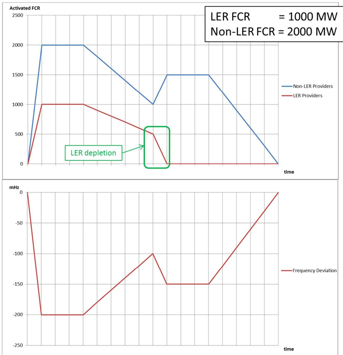
Figure 7: Acceptable situation - depleted LER can be replaced by non-LER
