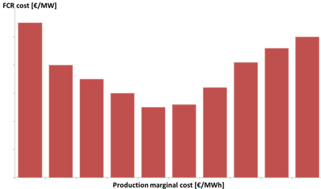
Figure 11: Dependence between FCR cost and variable cost for conventional plants
