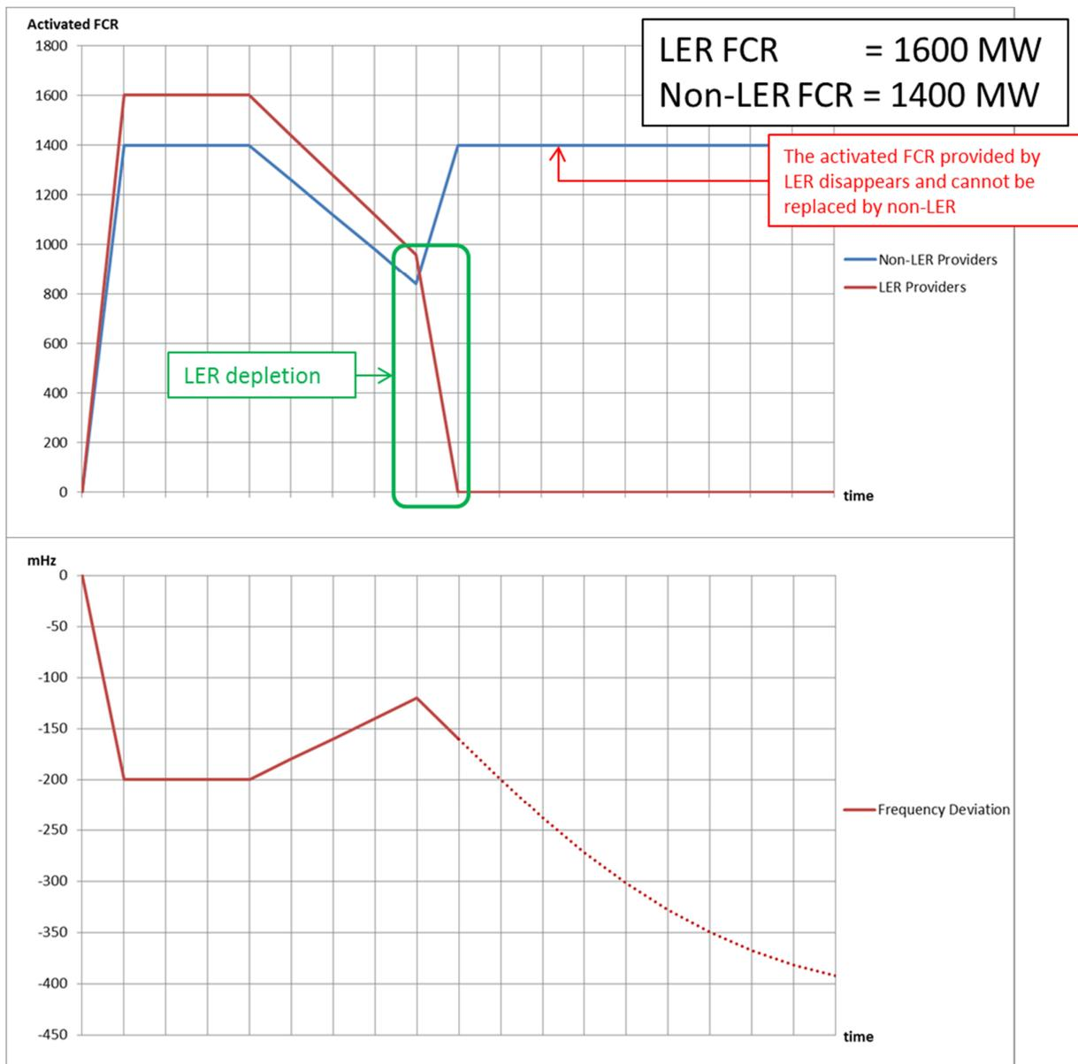
Figure 8: Not acceptable situation - depleted LER cannot be replaced by non-LER
