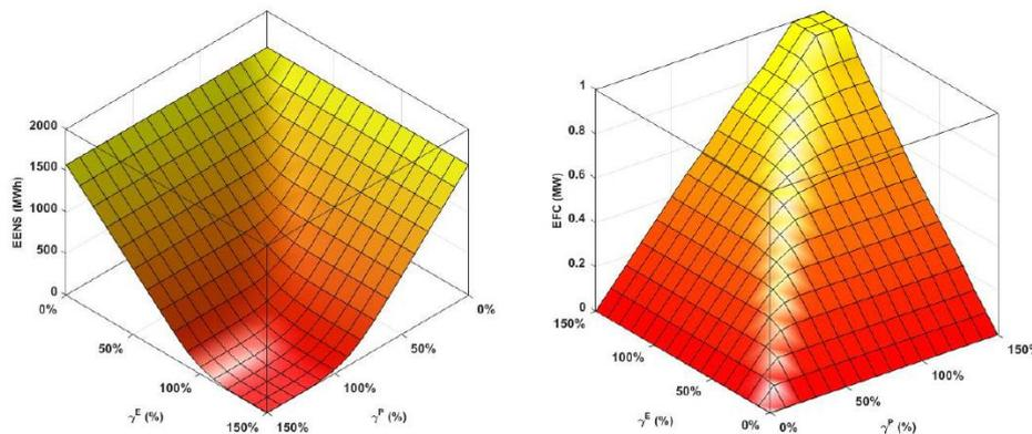
Figure 21: Sensitivity analysis of EENS and EFC as a function of power and energy allocation factors  $\gamma^P$  and  $\gamma^E$  under forecast errors  $\sigma^P = 20\%$  and  $\sigma^E = 20\%$ .
