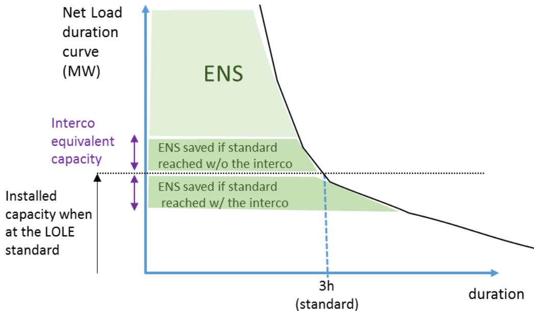
FIGURE 1 NET LOAD DURATION CURVE
