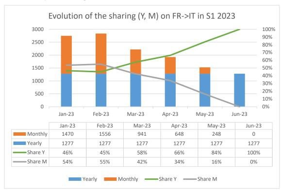
In the first semester of 2023, the link 2 of the new HVDC line between France and Italy has been commissioned. Therefore, the capacity has been added to the yearly computation in the last computation run in November 2022. The yearly capacity increased by about 100 MW but most of the capacity increase can be observed in the monthly timeframe especially in January with no reduction on the grid with an increase of about 200%. The behavior for February is also similar.
