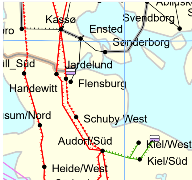
Figure 1: Topological overview of the Denmark West (DK1) – Germany (DE/LU) AC connection within CCR Hansa. Each red line represents a 380/400kV interconnector, consisting of a double circuit across the onshore border between Denmark (DK1) and Germany (DE/LU). The West Coast line from Klixbül to Endrup is not commissioned yet.
