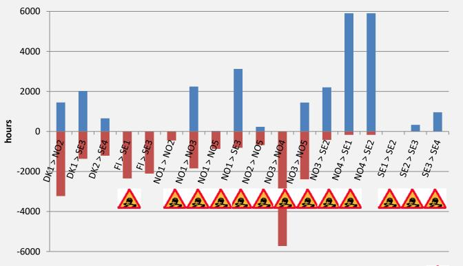
Number of hours in 2017 where a border capacity led to a price split due to thermal or dynamic limits.
